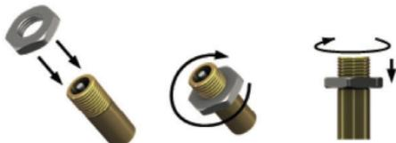
Screw the sensor onto the valve by hand and secure the sensor with the lock nut:
