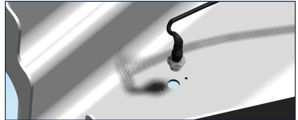
Next the fastening nut of the indicating LED must be tightened on the underside with 5 +3 Nm.
